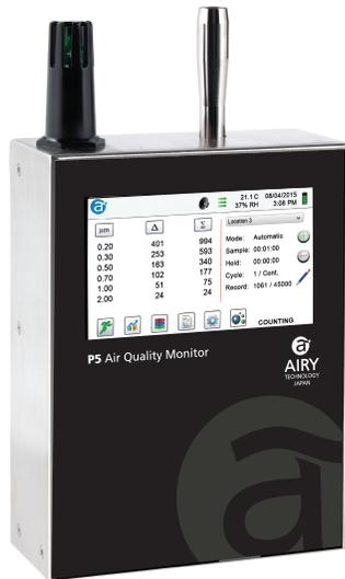
The Airy Technology Japan P5-30IP and P5-50IP Remote Particle Counters measure 0.3 or 0.5 to 25.0 µm with a flow rate of 0.1 CFM (2.83 LPM) from an internal vacuum pump and are the most feature-advanced remote particle counters available. Integration is easy into a building automation and cleanroom management system via Ethernet, or (optional) Wireless 802.11 b/g, RS485 or RS232
